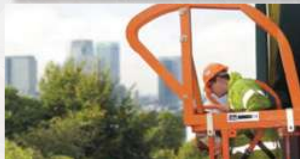
SanctuaryZone prevents the operator from being crushed
